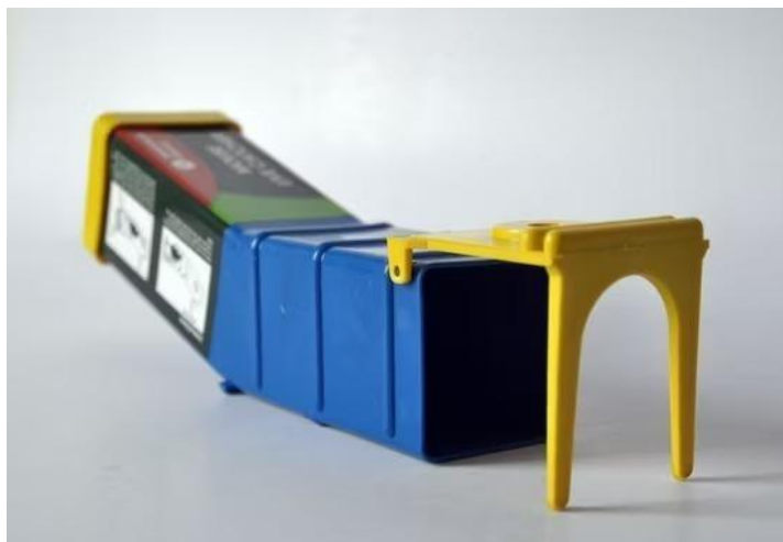
Figure 9: A humane tunnel-type live trap that uses a gravity-activated seesaw mechanism to capture House Mice ( Mus musculus Linnaeus, 1758) alive without toxic baits or physical injury
