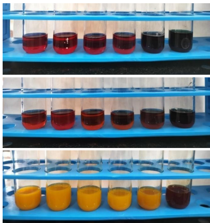
Figure 3: pH indicator test for dye extracted from rose, onion peel and turmeric at pH 2, 4, 6, 8 and 10.
