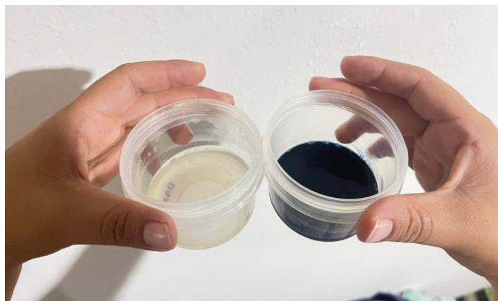
Figure 1: Reactions in a simple starch test when reacting with iodine as an indicator (deep navy blue color)
