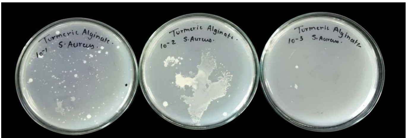
Figure 4A. Staphylococcus aureus - Petri plate images of S. aureus at serial dilutions ( 10^{-1} - 10^{-3} ) from turmeric-alginate film-coated slides
